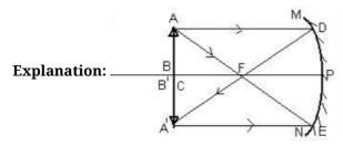
The ray diagram illustrates that, in the case of a concave mirror, the image size becomes equal to the object size when the object distance equals the radius of curvature, i.e, twice the focal length. So, the object has to be placed at a distance of  $(15\times2)=30$  cm in front of the concave mirror.
